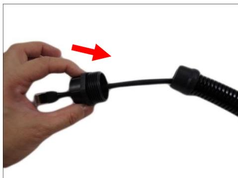
6. On the “pigtail” side, insert the washer into the “pigtail”.
