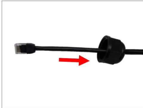
3. Insert the sealing insert with claw.
