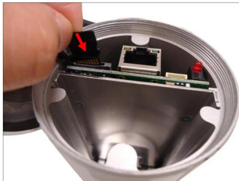
6. Before closing the back cover, make sure the Ethernet cable connector is connected to the main board. If the cable is disconnected, connect as shown below.
