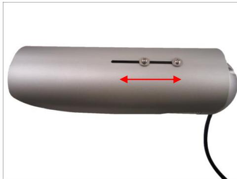
3. Tighten the screws to fix the position of the sunshield. See final installation below.
