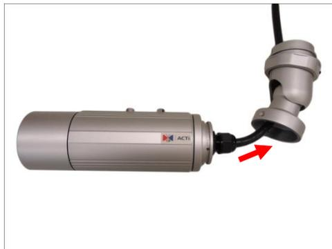
3. Remove the clamping nut and rubber insert to loosen the cable within the gland.
