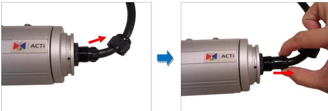
**NOTE:** Connectors are connected inside the camera, be careful when pulling the rubber insert from the gland.
