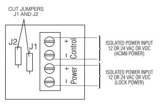
Fig. 3 Polarity reversal input from FACP signaling circuit output (polarity is referenced in alarm condition):
