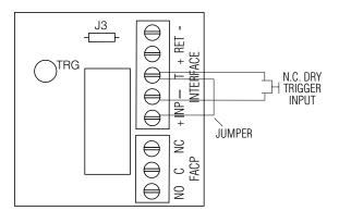
Fig. 7 Normally Closed - Latching FACP trigger input with reset:
