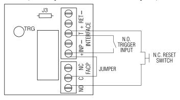
Fig. 6 Normally Closed - Non-Latching FACP trigger input:
