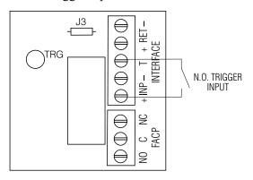
Fig. 5 Normally Open FACP Latching trigger input with reset:
