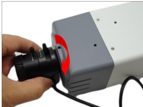
4. For lens with DC-iris, connect the lens cable to the DC-iris port of the camera.
