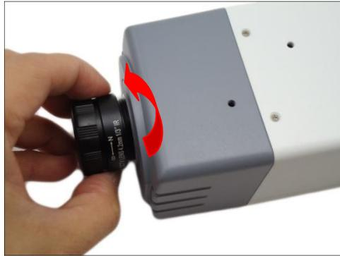
2. Twist and pull to remove the cap from the threaded end of the replacement lens.
