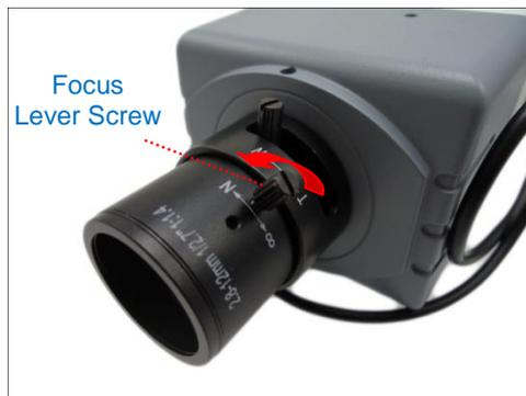
3. When done, tighten the lever screws to fix their position.
