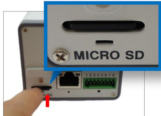
2. To avoid unauthorized removal of the card, cover the memory card slot. To do this, loosen the screw and turn the tab to cover the memory card slot. Once the tab is in place, tighten the screw.
