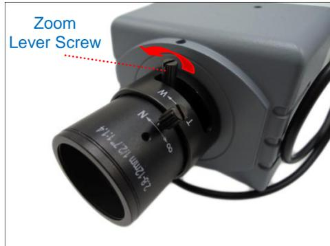
2. Loosen the focus lever screw, then turn left or right to adjust the focus.
