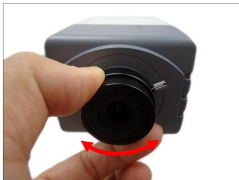
2. If necessary, tighten the lever screw to fix its position to avoid moving the lens.
