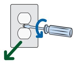
Hint - It's possible for the wall plate to be 'stuck' to the wall from being installed over wet paint or being painted over. This can sometimes peel paint from the wall when the wall plate is pulled off. To reduce the chance of paint damage, lightly score the corner where the wall plate makes contact with the wall.
