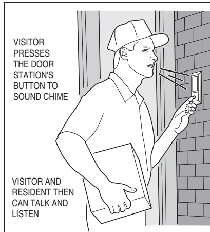
Figure 12. Door Station Operation
