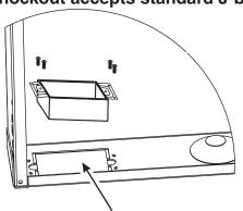
Remove rectangular knockout. Drop in J-box and attach with #6 sheet metal screws.
