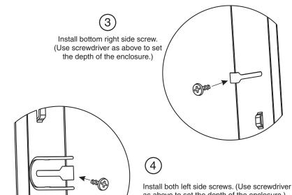
as above to set the depth of the enclosure.) The mount will flex to attach the enclosure to the stud without distorting the enclosure.
