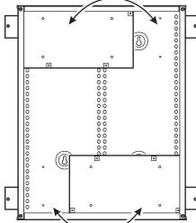
The H290/(H291) provides space for 4/(2) standard duplex receptacles. Wires should exit the H290/(H291) using the grommets provided. The grommets may be cut as shown.
