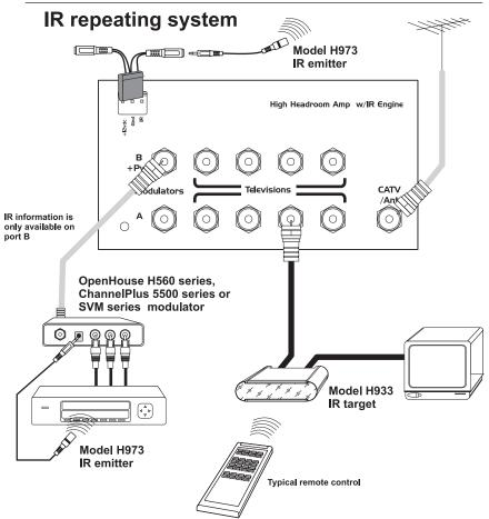
To control your video devices, add a modulator with IR repeating, an IR target and an IR emitter. Point a remote control at the target in the bedroom and IR pulses are repeated by the emitters, controlling the DVD player in the den.
