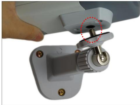
4. Tighten the hand knob until the camera is secured to the bracket.
