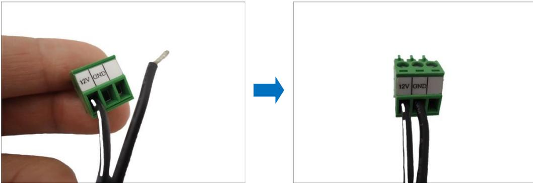
4. Tighten the screws of the **12V** pin and the **GND** pins to secure the wire connection.
