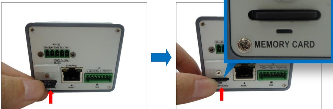
2. To avoid unauthorized removal of the card, cover the memory card slot. To do this, loosen the screw and turn the tab to cover the memory card slot. Once the tab is in place, tighten the screw.
