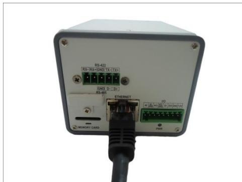
2. If necessary, connect a power adapter to the camera. See [Connecting a Power Adapter \(Optional\)](#) on page 19. Connect audio input/output or DI/DO devices to the camera. See [How to Connect DI/DO and Audio Devices \(Optional\)](#) on page 21.
