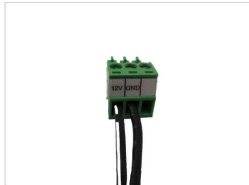
4. Tighten the screws of the **12V** pin and the **GND** pins to secure the wire connection.
