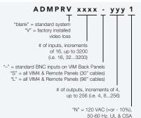
"N" = 120 VAC (+or - 10%), 50-60 Hz, UL & CSA "P" = 100-240 VAC, 50-60 Hz, CE
