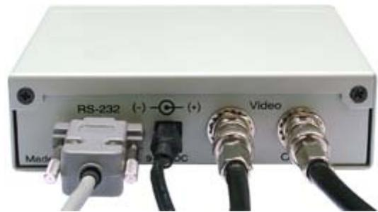
Serial Input    Power    Video Input    Video Output
