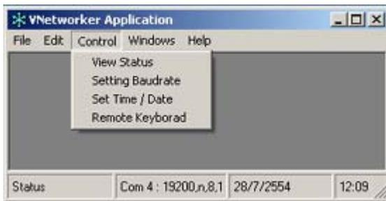
Figure 124: Vnetworker PC Software Main Menu
