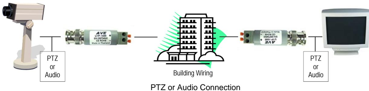
The AVE UTP-1500 module can be used as either a transmitter or receiver but is polarity sensitive. However reversing the wiring causes no ill effects to the device so if the picture is distorted just reverse the wires.
