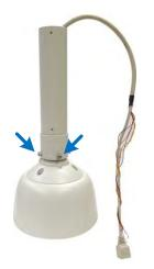
Thread the camera cable through the box cover (GV-Mount100, No. 2), assemble the box cover and the tube, and tighten the torxes with the supplied torx wrench (GV-Mount100, No. 7).
