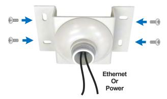
3. Assemble the tube (GV-Mount101, No. 2) and the tube connector (GV-Mount101, No. 3).
