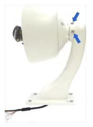
Thread the camera cable through the mounting bracket and secure the pendant tube to the mounting bracket. Slide the 30 mm M8 screws (GV-Mount400 / GV-Mount410, No. 3) from the front and secure from the backside using plain washer (GV-Mount400 / GV-Mount410, No. 5), split washer (GV-Mount400 / GV-Mount410, No. 6) and screw cap (GV-Mount400 / GV-Mount410, No. 7).
