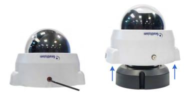
5. Align and secure the camera body to the wall mount bracket with three M3 screws (GV-Mount909, No. 4).
