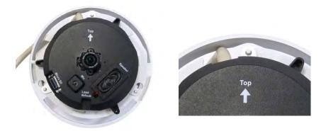
4. Secure the camera from the back with 3 long screws (GV-Mount904, No. 4).
