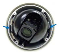
**IMPORTANT:** Be sure the desiccant is concealed in the GV-IP Speed Dome within 2 minutes of opening the desiccant pack.
