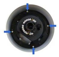
4. Secure the housing cap and the dome housing with M6 screws (GV-Mount902, No. 4).
