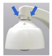
6. Hinge and hook the pendant tube to the junction box.
