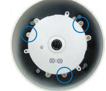
4. Place the camera cover for in-ceiling mount on the camera body and secure the 3 screws with the supplied torx wrench.
