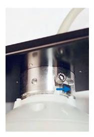
D. Put on another 2 screws (GV-Mount908, No. 4) and use the hex key (GV-Mount908, No.5) to secure all 4 screws tightly.
