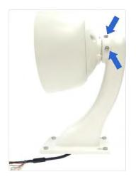
Thread the camera cable and secure the pendant tube to the plates. Slide the 30 mm M8 screws (GV-Mount903, No. 2) from the front and secure from the backside using plain washer (GV-Mount903, No. 3), split washer (GV-Mount903, No. 4) and secure with M8 screw cap (GV-Mount903, No. 5).
