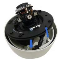
5. Thread the cable through the housing cap (GV-Mount901, No. 2) and secure with M6 screws (GV-Mount901, No. 4).
