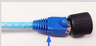
Unfit size of RJ45 Connector
