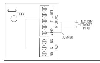
Fig. 8 Normally Closed - Latching FACP trigger input with reset:
