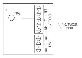
Fig. 6 Normally Open FACP Latching trigger input with reset:
