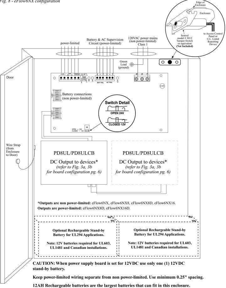
A UL Listed external battery enclosure must be used if using the 40AH or 65AH batteries.
