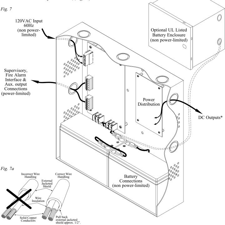
**\*Outputs are non power-limited:** eFlow6N, eFlow6N8, eFlow6N16. **Outputs are power-limited:** eFlow6N8D, eFlow6N16D.
