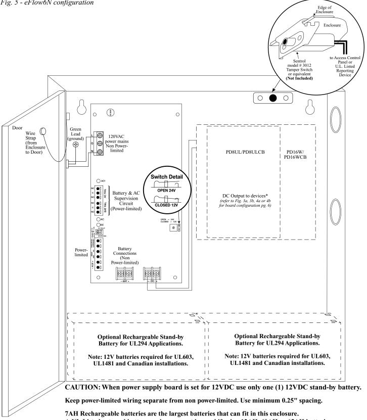
A UL Listed external battery enclosure must be used if using 12AH, 40AH or 65AH batteries.
