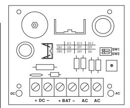
STEP 2: Mount SMP3 circuit board to nylon fasteners by pressing down circuit board onto nylon fasteners.
