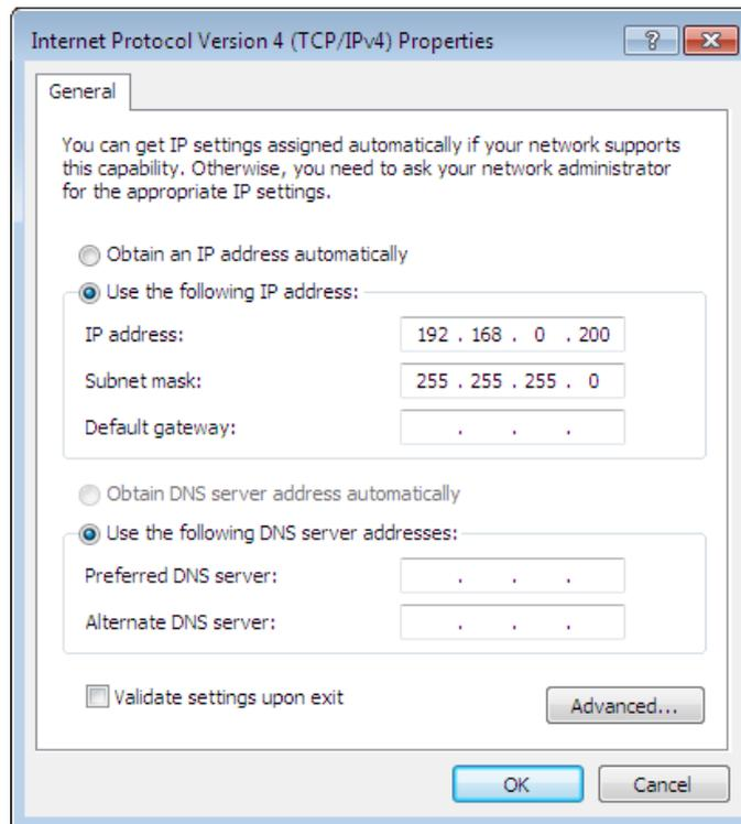
Figure 4-1 TCP/IP Setting
