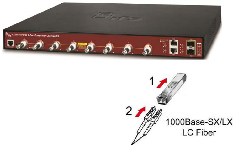
Figure 2-1-7 Plug in the SFP transceiver
