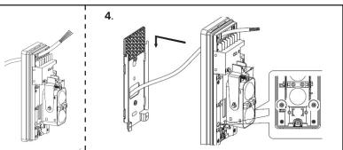
Figure 2.2: Inserting the wire and fastening the mounting plate to the sensor.
