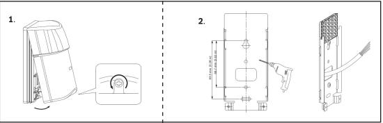
Figure 2.1: Fastening the mounting plate and removing the cover.
