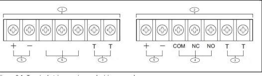
Figure 3.1: Terminal strip overview and wiring example.
