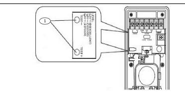
Figure 6.2: Using the test terminals
