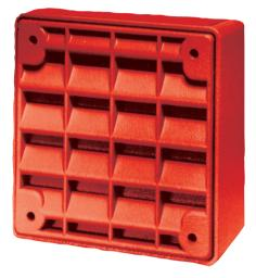
The Wheelock ET-1080-R Speakers meet the critical needs of the life safety industry for voice and tone signaling. They have a vandal-resistant die-cast grill and a sealed-back speaker for extra protection. The high-efficiency speaker is designed for multiple power requirements with high dBA output at each power tap. They provide a choice of field-selectable taps from 0.125 W to 8 W across a frequency range of 400 Hz to 4 kHz for either 25 V or 75 V audio systems.
