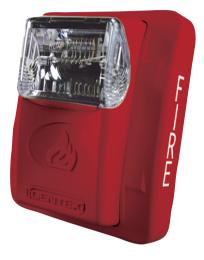
The Gentex GES24-15/75WR low-frequency strobe offers a dependable visual alarm, low current draw, 16 to 33 VDC or FWR voltage range, and a minimum flash rate of 1 Hz regardless of input voltage.
