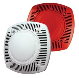
The G-SSPKCLP Low-profile Speakers are designed to meet code requirements for audio and voice communications. These speakers offer dependable evacuation signaling. They provide a 25 VRMS or 70.7 VRMS speaker with field-selectable power taps of 1/8 W, 1/4 W, 1/2 W, 1 W, 2 W, or 4 W.
