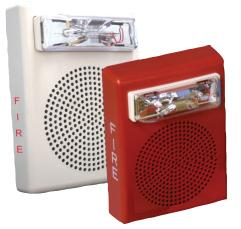
The Wheelock E50 Multi-candela Speaker Strobes meet the critical needs of the life safety industry for voice and tone signaling. They have high-efficiency sound output with dual voltage (25 VRMS or 70 VRMS) capability and field-selectable taps from 0.125 W to 2 W.
