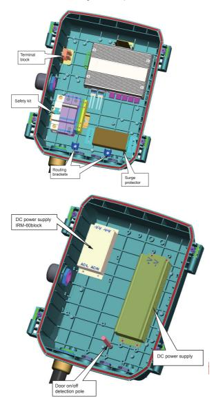
If fiber optics cables are used, install the cable holders for the bend radius concern.
