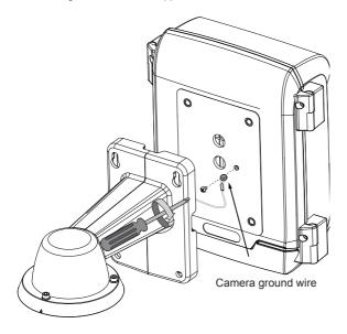
Connect all ground wires (including those from the surge protectors) to one position on the cabinet door, to the terminal block, and then to the external ground.
