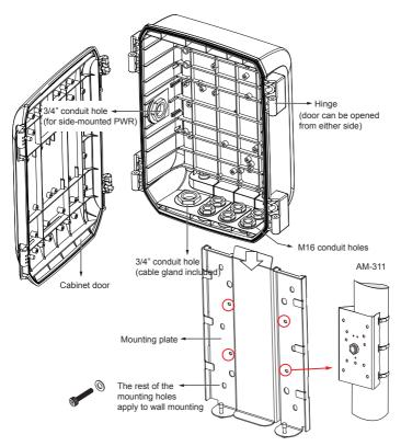
You can use the unused mouting holes for installing several cable clamps for routing the cables.
