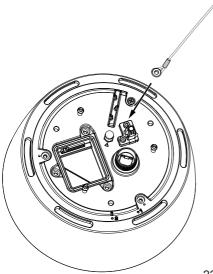
Connect the ground wire to the copper screw hole on the cabinet door.
