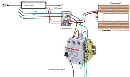
The surge protector becomes worn out after surges. When the indictor widnow changes color, replace the protecor. You can connect wires from its alarm terminal to a camera's DI pins so that you can receive notifications when the protector becomes worn out. Check the surge protector especially after lightning strikes. You can revceive the related alarm by configuring an event via Email, FTP, etc. via the
