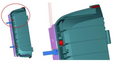
You can install one or two PoE switch, media converter, or industrial power supply to the vertical DIN rail. Please refer to page 2 and page 3 for information.
