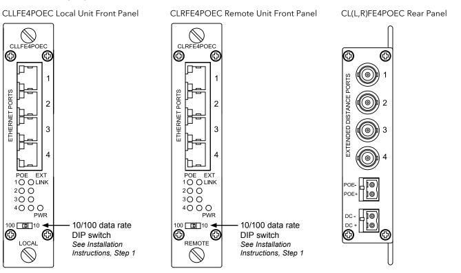
FIGURE 9 - CL(L,R)FE4POEU FOUR CHANNEL SURFACE OR RACK MOUNT UTP UNIT
