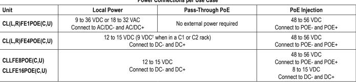
Note: Use only one of the two power connectors, based on the power requirements of your application.
