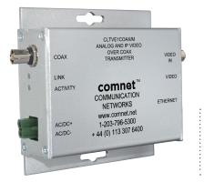
The ComNet<sup>™</sup> CL(T,R)VE(1,2)COAX[POE][/M] is a communications link that combines composite analog baseband video and 10/100T(X) Ethernet on a single RG59 coaxial cable and transmits it up to 500 meters. The device is particularly suited to applications where the addition of IP Video to an existing analog video system is required. The CLTVE1COAXPOE/M model can provide power to the IP device via PoE.
