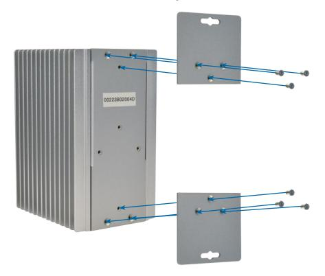
Step 4: Repeat Steps 2 and 3 to mount the second wall mount panel on the bottom of the unit's back panel.
