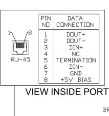
NOTE: A 120 DHM TERMINATION RESISTOR IS APPLIED TO THE DIFFERENTIAL INPUTS WHEN "TERMINATION (PIN 5)" IS WIRED DIRECTLY TO "DIN- (PIN 6)" SEE DIAGRAM BELOW
