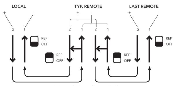
Figure 10. 2-Wire RS-485 Local/Remote Configuration HD is selected on all Link/Repeaters All IEDs have the ability to hear and respond to each other.
