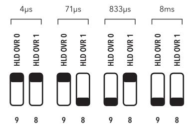
Figure 4. Enable Holdover Switch Settings
