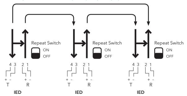
FIGURE 12. Peer-to-Peer Loop Configuration
