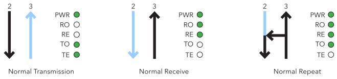
Figure 6. Diagnostic LED patterns and signal paths
