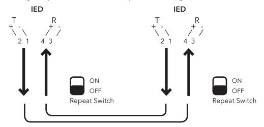
Figure 7. Point-to-Point Configuration
