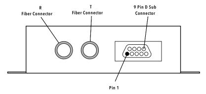
Figure 5 Optical Ports and Electrical Port
