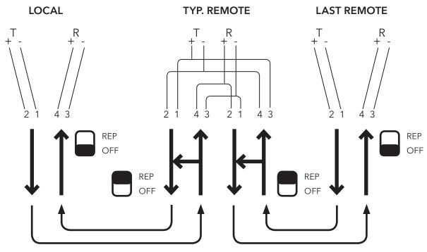
Figure 9. 4-Wire RS-485 Local/Remote Configuration FD is selected on all Link/Repeaters All Remotes hear the Local's Poll. Only the Local hears the response.
