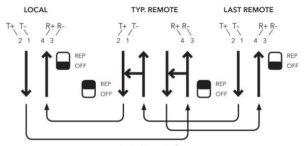
Figure 8. RS-422 Bus Configuration FD is selected on all Link/Repeaters All Remotes hear the Local's Poll. Only the Local hears the response.
