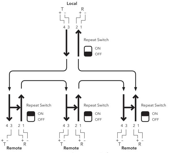
Figure 11. Local/Remote Loop Configuration
