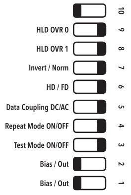
Figure 3. Switch Settings (Factory Defaults)
