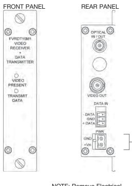
NOTE: Remove Electrical Connector for Rack Mount Units
