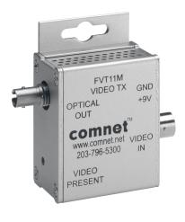
The ComNet™ FVT11M video mini-transmitter supports transmission of a fixed video signal using AM modulation on one multimode fiber optic cable. The FVT11M video transmitter is compatible with the FVR11M, FVR10M, FVR21, and FVR22 receivers. Plug-and-play design ensures ease of installation requiring no electrical or optical adjustments. The transmitter incorporates a bi-color (Red/ Green) indicating LED for monitoring proper system operation.
