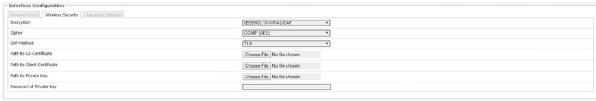
Figure 45: Encryption options for WPA-EAP or WPA2-EAP in Client mode.
