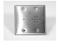
**STW1** Two Way Microphone / speaker Omni-directional pre-amplified microphone and speaker for use in two way surveillance systems.
