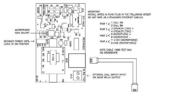
**CONNECTIONS TO MSI-BOC5 (SEPARATE MICROPHONE AND SPEAKER)**
