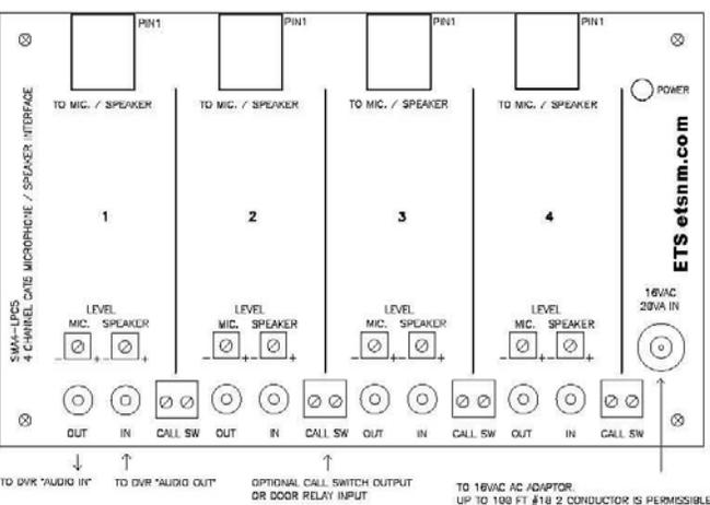
**CONNECTIONS TO MSI-C5 (CSMB AND HSM11)**
