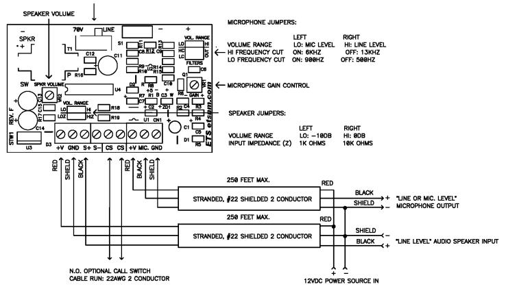
LINE/MIC. MICROPHONE OUTPUT AND LINE LEVEL SPEAKER INPUT
