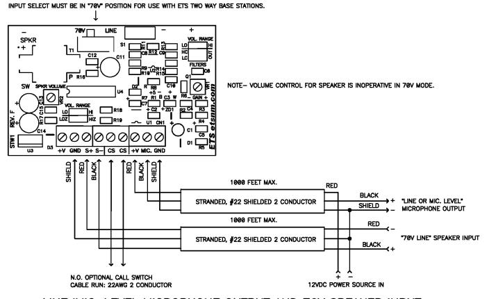
LINE/MIC. LEVEL MICROPHONE OUTPUT AND 70V SPEAKER INPUT
