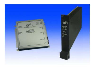
The American Fibertek 46 Series transmits and receives (2) copper 10/100 BaseT Ethernet signals at the RJ45 ports and (1) optical 100 Base-FX over 1 or 2 multimode fibers. The system is comprised of two units forming a point-to-point communications link.
