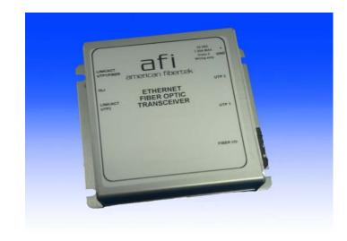
The American Fibertek 46SL-PoE+ Series transmits and receives (2) copper 10/100/1000 Base-T Ethernet signals at the RJ45 ports and (1) optical 100 Base-FX over 1 or 2 singlemode fibers. The system is comprised of two units forming a point-to-point communications link.
