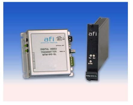
The American Fibertek M910SL Series transmits one channel of highquality 10 bit digitized video on one singlemode optical fiber over a distance of up to 40 km. The receiver rack cards are available in a single channel M910SL or a two channel M920SL configuration. The M920SL utilizes 2 fibers, one for each channel.
