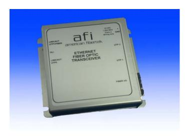
The American Fibertek 46-SL-PoE-HP Series transmits and receives (2) copper 10/100 Base-T Ethernet signals at the RJ45 ports and (1) optical 100 Base-FX over 1 or 2 singlemode fibers. The system is comprised of two units forming a point-to-point communications link.
