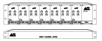
The American Fibertek 95600C-SL Series transmits 56 channels of high-quality 10 Bit digitized video on one singlemode optical fiber using CWDM technology.
