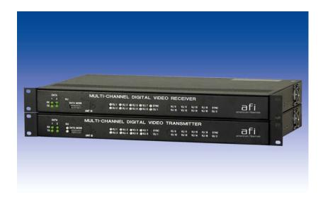
The American Fibertek 91685C-SL Series transmits 16 channels of high-quality 10 Bit digitized video and two channels of multi-protocol data on one singlemode optical fiber using WDM technology.
