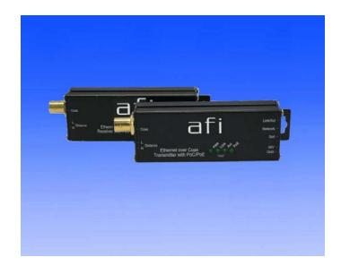
The American Fibertek Series SLC-1-PoE EoC solution allows for the utilization of existing coax cable infrastructure to transmit bi-directional data from IP cameras and other network devices. The AFI Series SLCR-1-PoE receiver power supply provides Power Over the Coax (PoC) to power the SLCT-1-PoE transmitter which also provides PoE to the IP camera. The PoE power supply is ordered separately.
