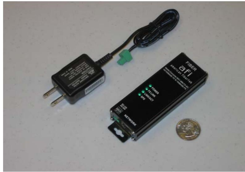
The American Fibertek MTX1M-FX and MRX1M-FX Series transmits and receives 10/100 Base-TX Ethernet signals at the RJ45 port and 100 Base-FX at the optical port over one or two, multimode or singlemode, fibers. The system is comprised of two units (MTX1M to MRX1M) forming a point-to-point communications link.
