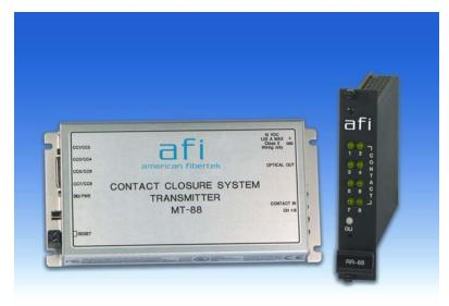
The American Fibertek 88 Series multiplexes 8 channels of "supervised input" dry contact closure on one multimode fiber. A set of 8 LEDs on the transmitter and the receiver units indicates the channel(s) status.
