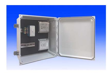
The American Fibertek Enclosure Kit *ENC-1W* provides a complete set of components for assembling *American Fibertek field devices in secure weatherproof installations.* The enclosure kit includes a base plate which accommodates *most afi* modules *and has been drilled and tapped for easy mounting* (screws included), DIN rails (top hat rail EN 50022 – 35mm x 7.5mm), and DIN rail mounted power supply connectors.
