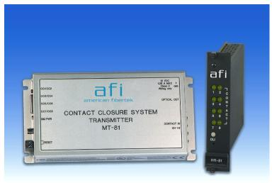
The American Fibertek 81-280 Series multiplexes 8 channels of dry non-latching contact closure on one multimode fiber. Both normally open and normally closed outputs are available. A set of 8 LEDs on the transmitter and the receiver units indicates the channel(s) status.
