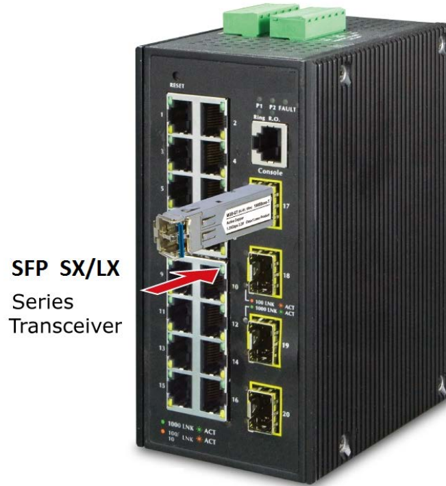
Figure 2-25: Plug in the SFP Transceiver
