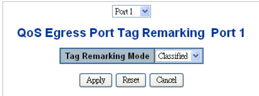
Figure 4-9-7: QoS Egress Port Tag Remarking page Screenshot
