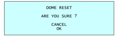
This feature is used to re-calibrate the orientation of a selected dome camera. Origin offset value is not affected by this function. (Offset is still valid after origin set.)
