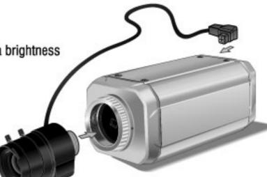
Remove the lens mount cap from the camera.
