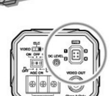
Please attach a lens cable when using the DC iris lens or Video iris lens.
