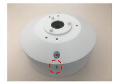
8. Align the two screw holes of the camera with the screw holes on the pole mount junction box cover and fasten the camera with the M4 machine screws. The drainage hole should point down when installing horizontally.
