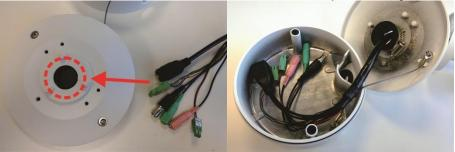
4. Insert the rubber plug back to the cable entry hole and use a flathead screwdriver to tighten the stainless steel ring by turning the knob clockwise. Make sure there's no gap between the All-In-One cable and cable entry hole.
